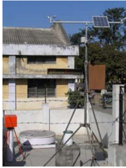
Automatic Weather Monitoring System installed Patiala (Punjab) , India
