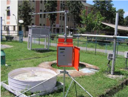
Pyranometer with Albedo installed at NIH, Roorkee (UA) India
