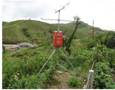
Automatic Weather Station installed at Cherapungi (Meghalaya) , India
