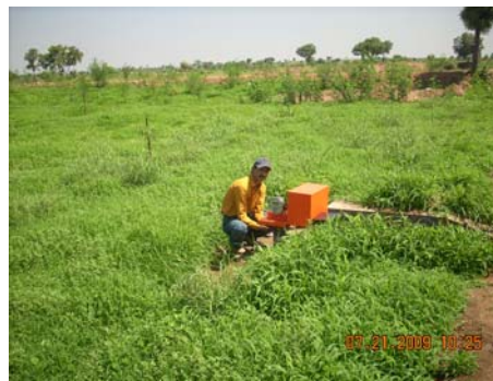
Automatic Water Level Recorder installed at Jhansi (UP)
