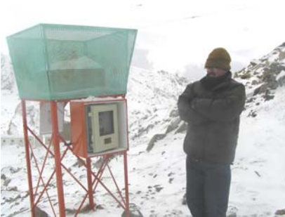
Automatic SWE Recorder installed at Leh (J&K), India
