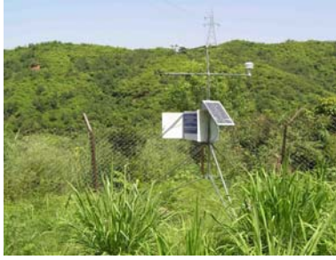
Automatic Weather Station with Data Logger installed at Jammu, J&K, India
