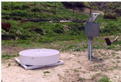
Automatic Evaporation Rate Recorder with Data Logger installed at , Qazi Kund, Anantnag J&K, India
