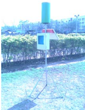
Digital Rainfall Recorder installed at Bhubeneshwar (Orissa) Automatic Weather Station installed at Srinagar (Uttarakhand) India
