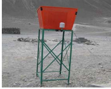
Automatic Snow Water Equivalent Recorder with Data Logger installed at NHPC, Leh (J&K), India by our dealer
