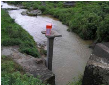
Automatic Water level Recorder installed at (Cherapuji) Meghalaya, India
