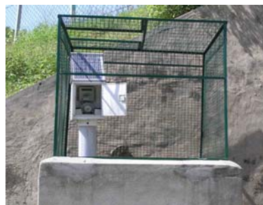
Automatic Water Level Recorder with Data Logger installed at Ragoora Nala, Jammu, J&K, India
