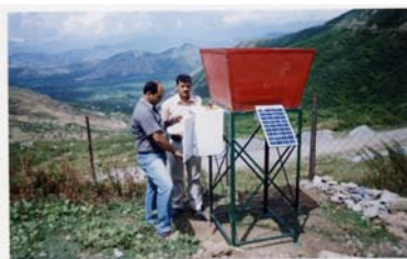
Automatic Snow Water Equivalent Recorder with Data Logger installed at Khaji gund, J&K, India
