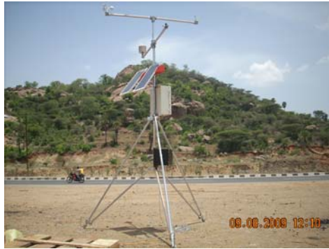
Automatic Weather Station installed at Nammakal Tamilnadu, India
