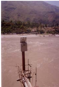
Automatic Water Level Recorder with Data Logger installed at SJVNL Himachal Pradesh, India by our dealer
